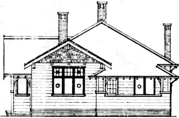
Frethey bungalow west elevation. Front porch on left, sleeping porch on right
